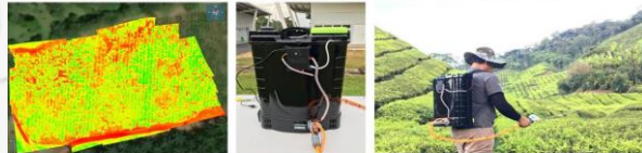
Product integration with GPS-guided automated fertilizer dispenser backpack for IoT agriculture application
