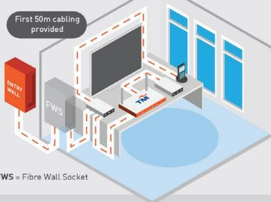
FWS = Fibre Wall Socket
