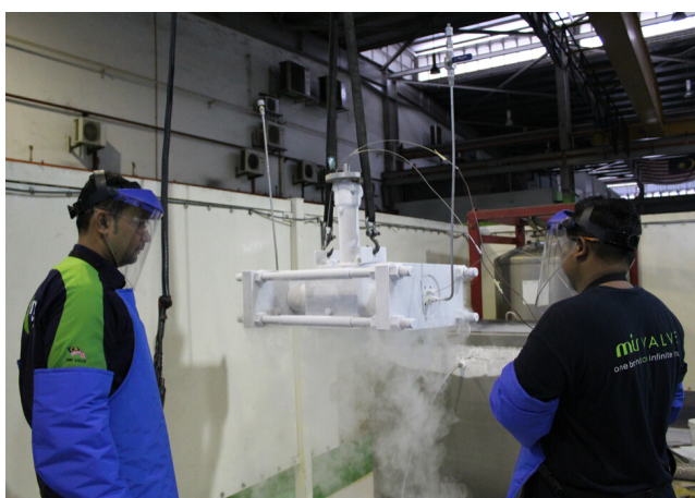
In-house Cryogenic Testing at -196°C
